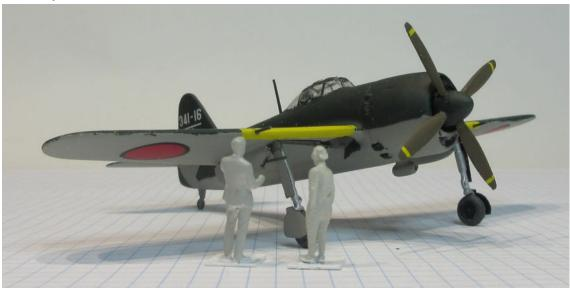
Despite its superior performance the N1K1-J had temperamental flight characteristics that required an experienced pilot. It also suffered from engine reliability problems, was complex to manufacture and had long, weak undercarriage because of the mid-fuselage location of the wings.
